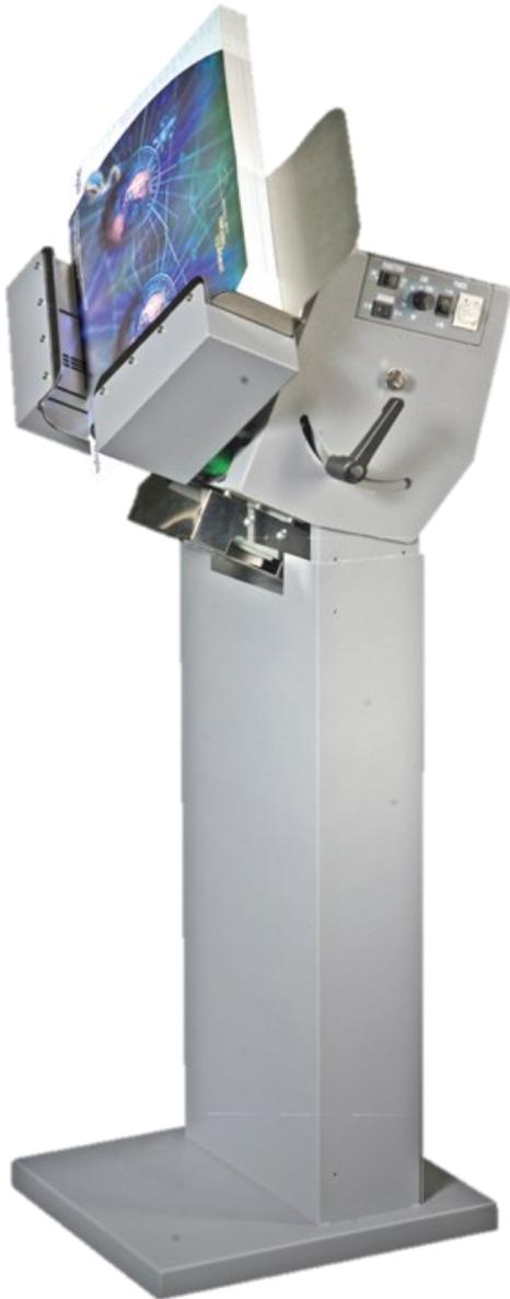
The UJ-500AS Paper Air Jogger maximizes prints jogging efficiency for digitally printed documents before being used into finishing equipment: collators, feeders, coaters, folders, cutters and many more. The ionized air-assisted blowing power helps eliminating static generated by upstream printing equipment and prevents machine downtime.
